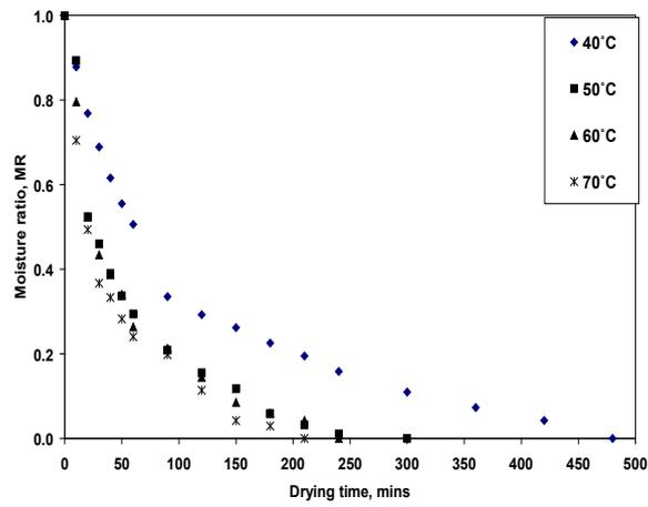
Figure 4. Moisture ratio for EX-BORNO millet
